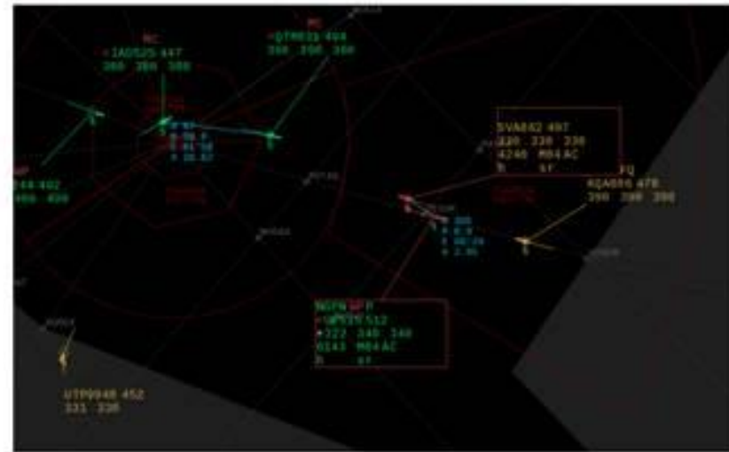
Figure showing breach of separation between SVA862 and UPS15
