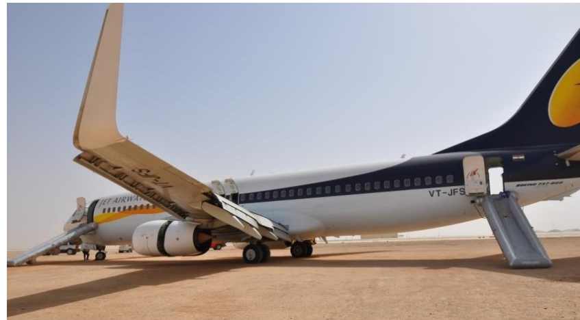
Position of the final stop of aircraft VT-JFS showing the emergency escape slides deployed on an unpaved ground
